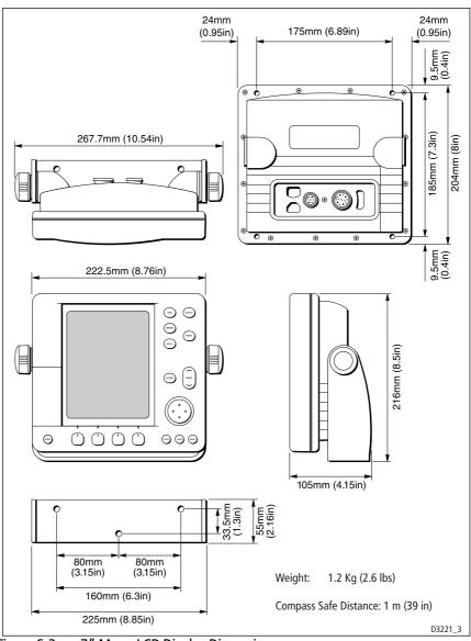
Figure 6-3: 7" Mono LCD Display Dimensions
